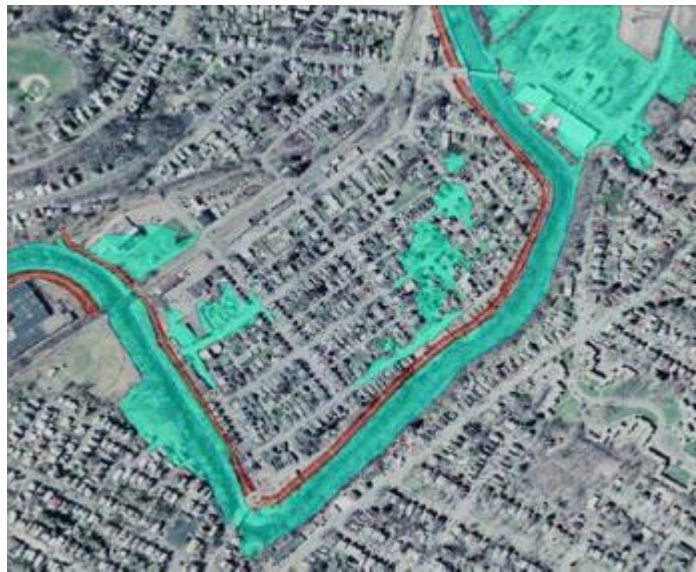
USACE floodplain delineation and inundation mapping
